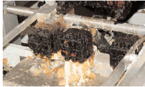
Glue nozzles in a food packaging plant before and after Dry Ice Cleaning
